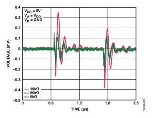
Figure 32. Digital Feedthrough
