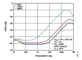
Figure 31. Power Supply Rejection Ratio (PSRR) vs. Frequency
