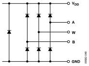
Figure 49. Maximum Terminal Voltages Set by V<sub>DD</sub> and GND
