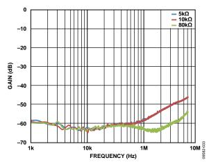
Figure 33. Shutdown Isolation vs. Frequency
