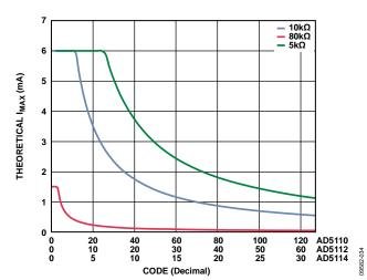
Figure 34. Theoretical Maximum Current vs. Code
