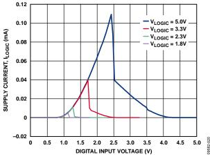
Figure 20. Supply Current (I<sub>LOGIC</sub>) vs. Digital Input Voltage
