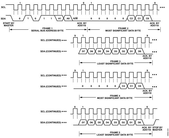
Figure 44. AD5110 Interface Multiple Write
