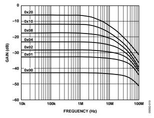
Figure 19. 5  $k\Omega$  Gain vs. Frequency vs. Code
