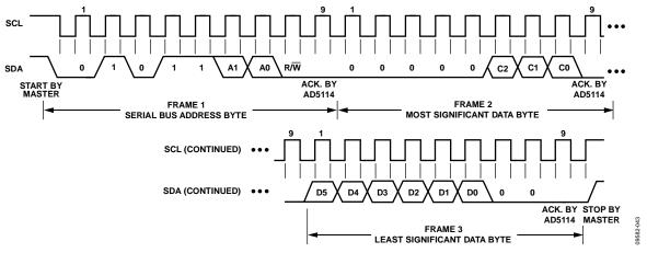
Figure 43. AD5114 Interface Write Command
