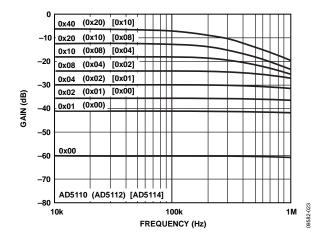
Figure 23. 80 k $\Omega$  Gain vs. Frequency vs. Code
