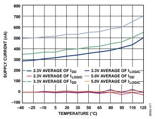
Figure 17. Supply Current vs. Temperature
