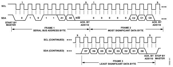
Figure 41. AD5110 Interface Write Command
