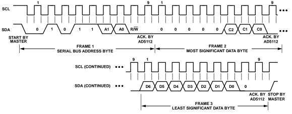
Figure 42. AD5112 Interface Write Command
