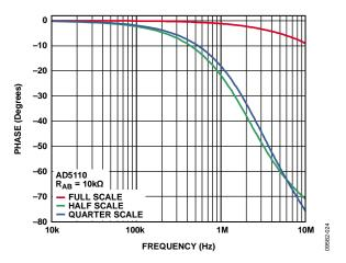
Figure 24. Normalized Phase Flatness vs. Frequency
