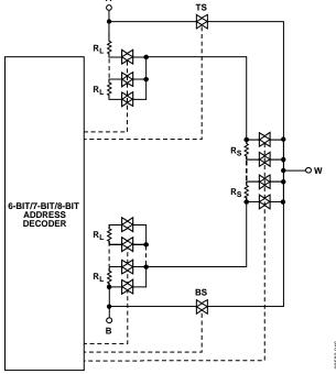
Figure 46. AD5110/AD5112/AD5114 Simplified RDAC Circuit
