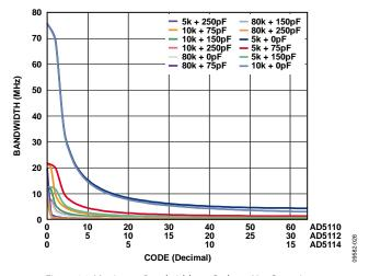
Figure 26. Maximum Bandwidth vs. Code vs. Net Capacitance
