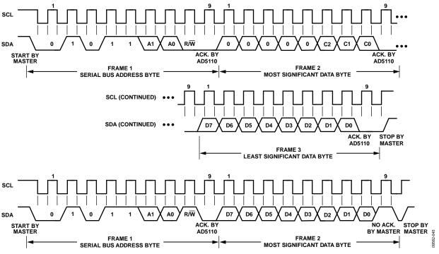
Figure 45. AD5110 Interface Read Command
