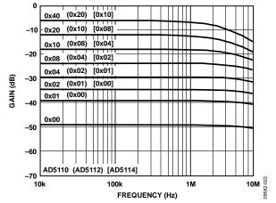
Figure 22. 10 k $\Omega$  Gain vs. Frequency vs. Code
